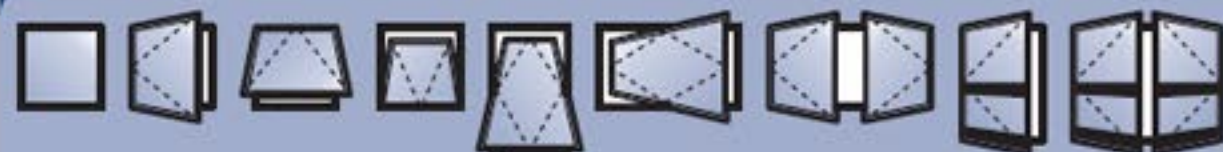
fixed light Side hung Top hung Bottom hung Horizontal pivot Vertical pivot Folding double Single door Double door All side hinged casements and doors can open either inwards (open in) or outwards (open out).
