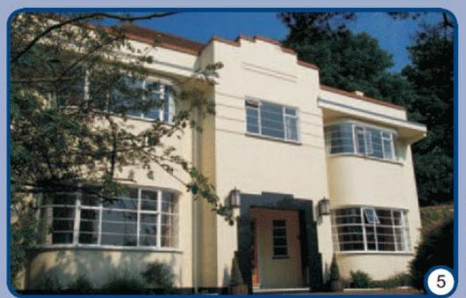
5. SMW "F" series windows with horizontal "true" 19mm steel glazing bars in a white polyester powder coating
